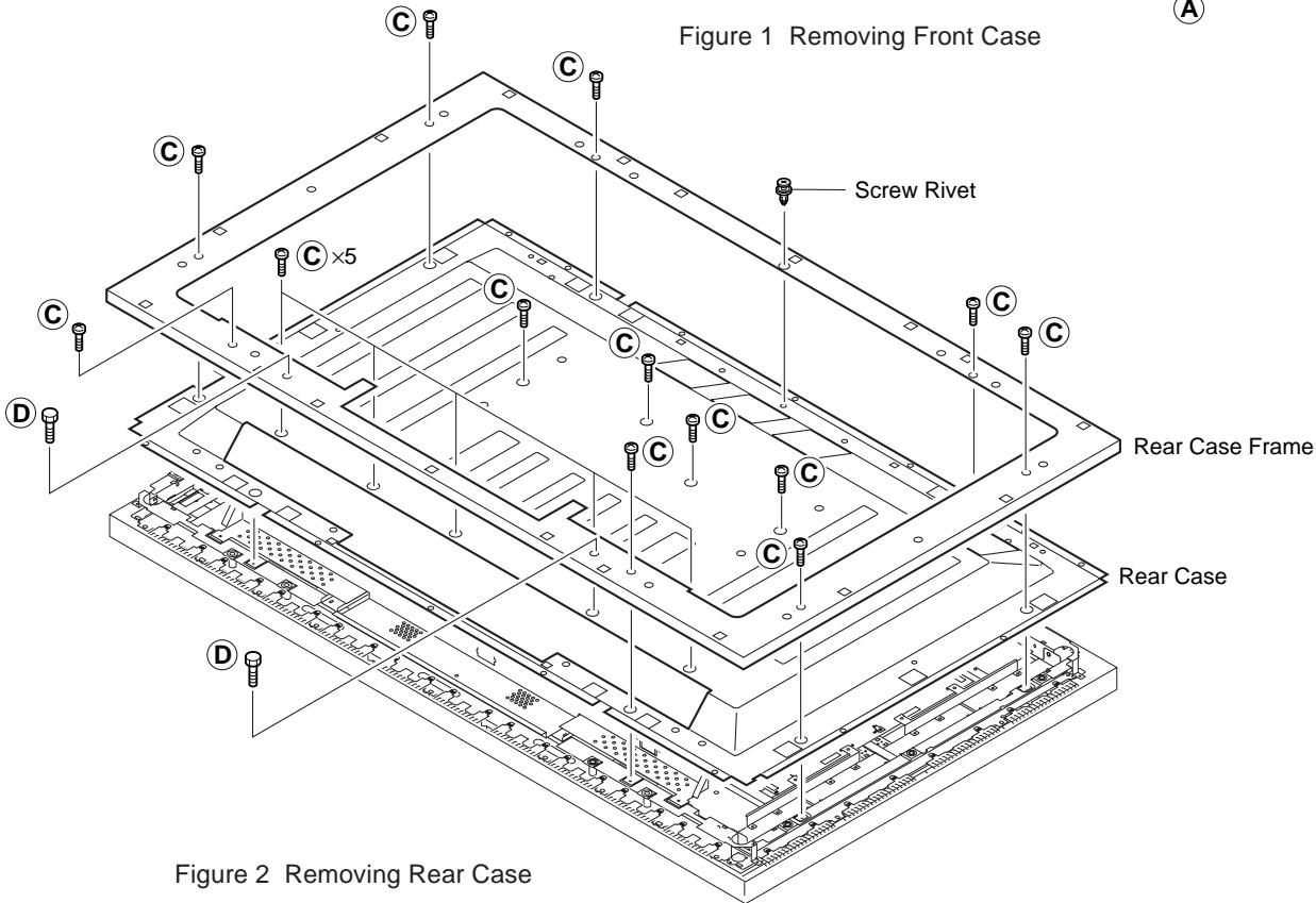
Figure 2 Removing Rear Case
